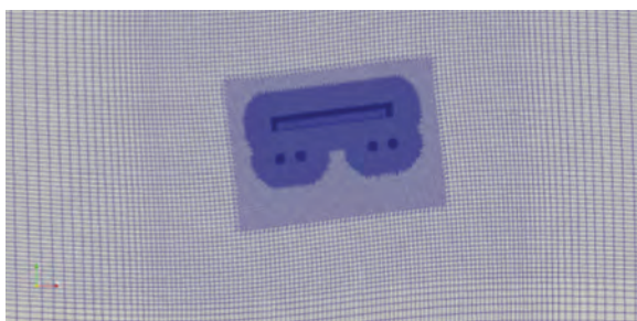
Figure 11 Example of mesh refinement for 2M, 4M and 6M of the pitch decay simulation in OpenFOAM
